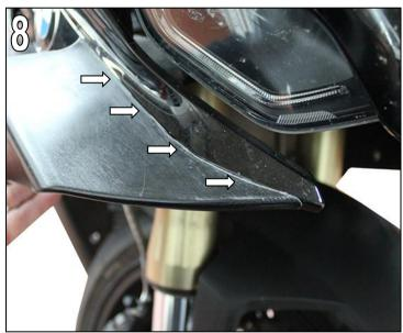
**Fig. 9**Make sure that the contour in the rear area of the AC Schnitzer winglets is flush with the side panel.
