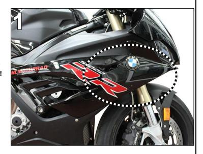
Fig. 2 Stickers that have not been painted over must be removed before fitting the AC Schnitzer winglets.
