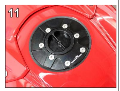
Check the fastening screws for tightness.
