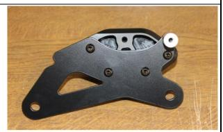
Loosen and remove both engine mounting screws on the left-hand side (these will not be reused).
