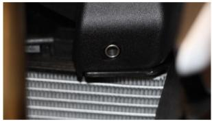
Loosen the left and right trim, pull it out of the retaining pegs and remove.
