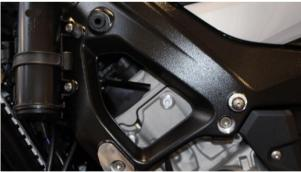
Loosen and remove both engine mounting screws on the right-hand side (these will not be reused).
