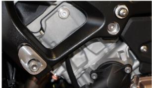
Insert the supplied spacer sleeves into the frame. Secure the crash pad to the frame with the washers and screws supplied. *Same meaning as on the right side.*
