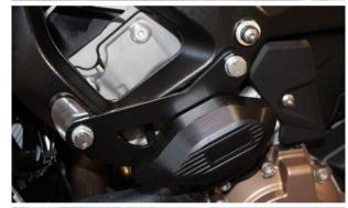
Clean the recess in the pad and stick in the sticker. Press the plastic covers onto the right-hand screw head.
