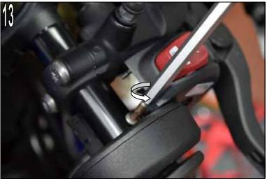
Completely screw in the adjustment screw of the clutch cable on the left side of the vehicle.
