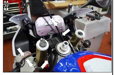
Remove the ignition lock from the standard triple clamp. To do this, drill a hole into the shear bolt, drive in the Torxbit and remove the bolts.
