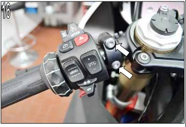
Fold away handle lip, loosen exposed fastening screw with Torx screwdriver and remove.
