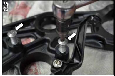
Fasten the standard ignition lock to the supplied AC Schnitzer triple clamp as shown in the illustration using the supplied fixing screws and sleeves.
