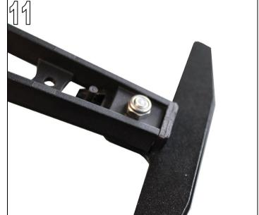
Refit the number plate holder incl. licence plate and the **3 rubber washers** supplied to the vehicle.
