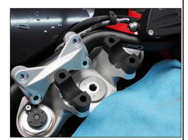
Insert the supplied AC Schnitzer handlebar risers into the fork bridge lower part of the clamping hole.
