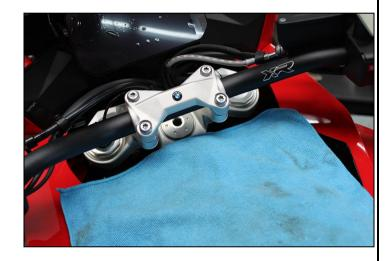
Loosen the four fixing screws of the handlebar clamp anti-clockwise.
