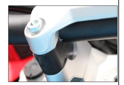
Tighten the handlebars incl. handlebar clamp.
