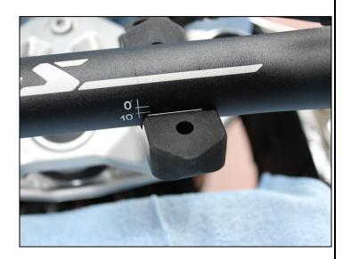
Apply "medium-strength" threadlocker to the standard fastening screws and screw them in.
