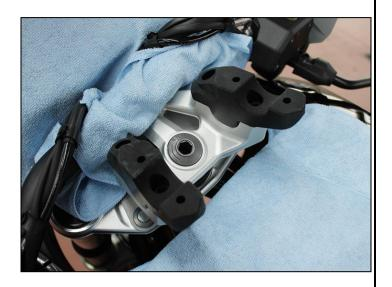
Insert the supplied AC Schnitzer handlebar risers into the fork bridge/clamping hole bases.
