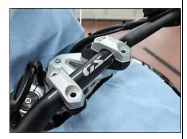
Tighten the handlebars incl. handlebar clamps.
