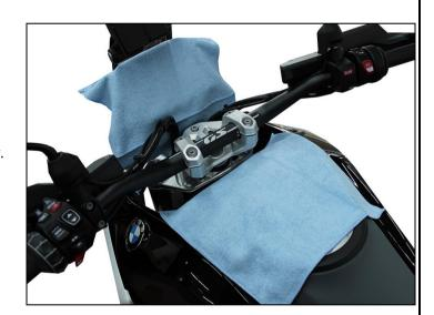
Loosen the four fixing screws of the handlebar clamps anti-clockwise.
