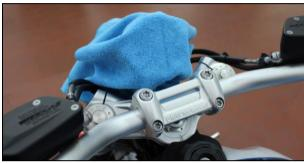
Loosen the four fastening screws of the handlebar counterclockwise and remove it.
