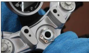
Note the markings R (right) and L (left) on the handlebar risers. handlebar risers.
