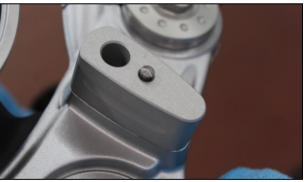
Place the original clamp bases on the handlebar riser. on the handlebar riser.
