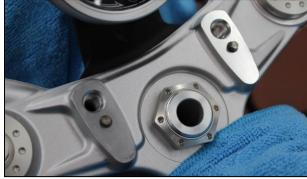
Insert the supplied AC Schnitzer handlebar risers into the standard cylindrical pins of the triple clamp.
