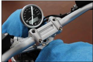
Place the upper part of the clamp and screw in the prepared screws hand-tight.
