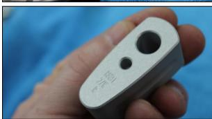
Insert the two enclosed dowel pins into the handlebar riser. into the handlebar riser.
