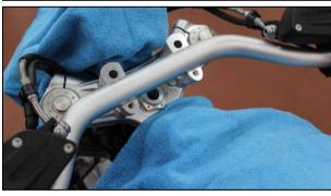
Remove the handlebars from the triple clamp and store them in a place protected against damage.
