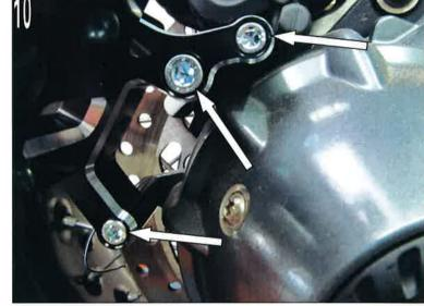
Fit the mounting screws of the licence plate holder with the supplied cover caps.
