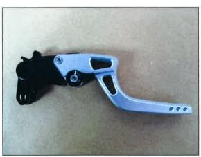
AC Schnitzer EVO brake & clutch lever (with ABE) S700-68779-63
