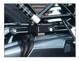
AC Schnitzer Paralever brace, adjustable (with TÜV parts certificate)
