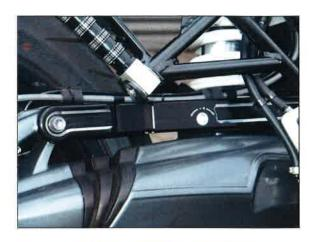
AC Schnitzer Paralever brace, adjustable (with TÜV parts certificate) S700-68789-15
