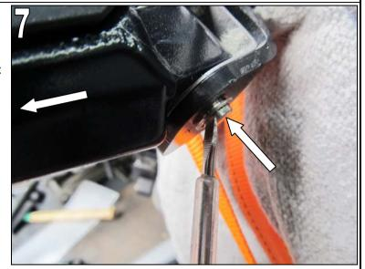
Remove retaining plate from standard footrest.WARNING! Do not lose the spring or locking ball!Clean parts and check for perfect condition (Fig.
