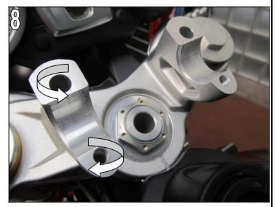
Loosen the right & left fixing screws of the fork bridge clamp on the upright by approx. 2 turns. (Fig. 9).
