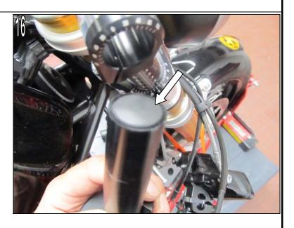
On both sides: - Push handlebar stumps flush into stump holder. (Fig. 17)
