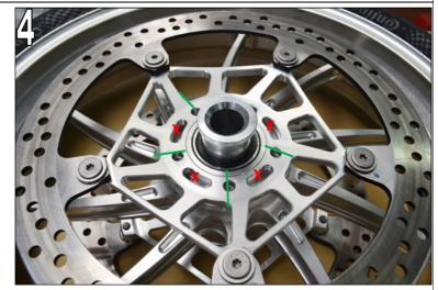
Place the spacer ring "A" supplied on the cleaned, untreated and uncoated brake disc adapter. Make sure that the bore holes (~8mm) are congruent with those of the brake disc adapter.
