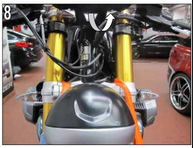
Tilt back headlamp, align to standard dowel pins, and secure with standard bolts (M6 x 20).
