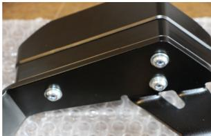
Insert the enclosed short spacer sleeves into the frame. Lightly grease the screw thread.
