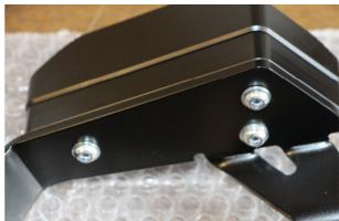
Insert the enclosed spacer sleeves (with the smaller diameter facing inwards) into the frame.
