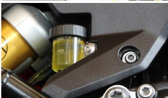
Attach the enclosed holder with the O-rings, screws and washers to the AC Schnitzer Brake fluid reservoir (see picture).
