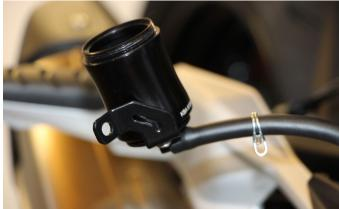
Push the original brake fluid hose onto the reservoir connection fix it with the safety clip.
