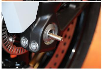
On the left side, fit the pad with the washer and nut. nut.
