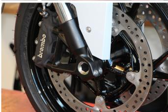
Push the pre-assembled pad with the threaded rod from the right through the axle.
